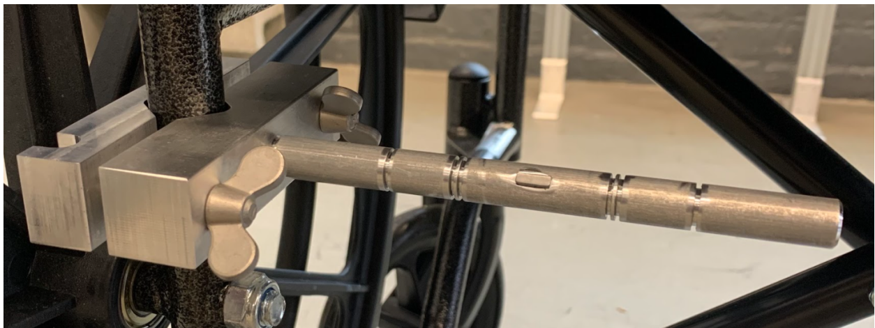
Figure 29 : Wing nuts used in an older design iteration that could be tightened by hand but did not provide enough force to fix the attachment.
