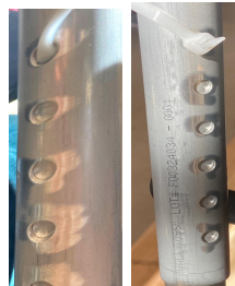
Figure 32. Spring rod attachments connected using zip ties
