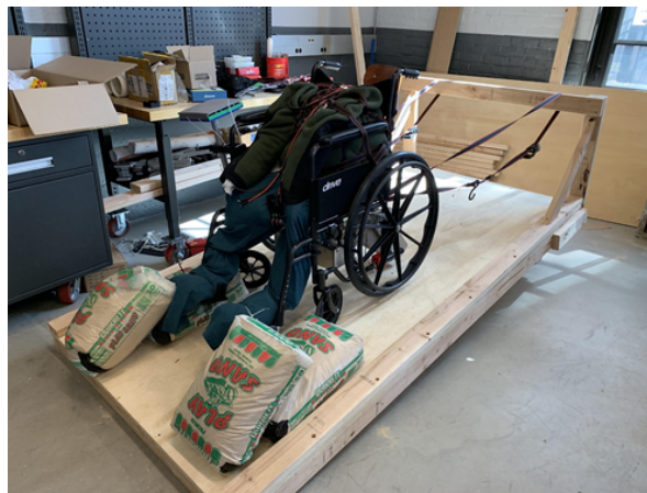
Figure 21 Adjustable test ramp with test dummy and wheelchair on ramp
