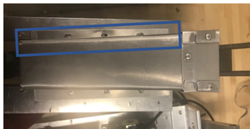
Figure 30: Spring Housing not aligning with tapped holes on base plate due to imperfect bending and complexity of design
