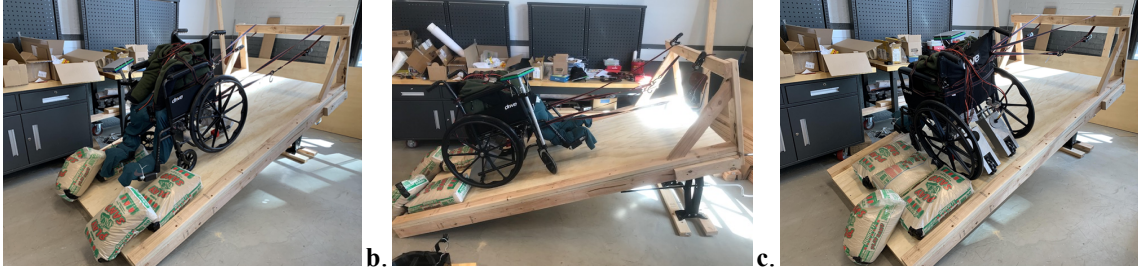
Figures 25a 25b & 25c Static Stability test at maximum angle in the backwards (a), forwards (b) and lateral (c) orientations
