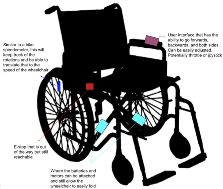
Figure B.9 Option for where we can place batteries, Estop, user interface and speedometer [5, modified]
