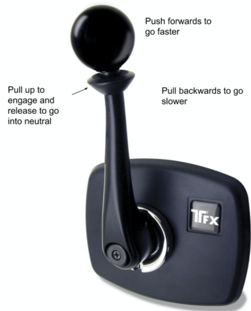
Figure B.10 (a) Placement of throttle (b) Throttle with description of mechanism [30, 31, modified]
