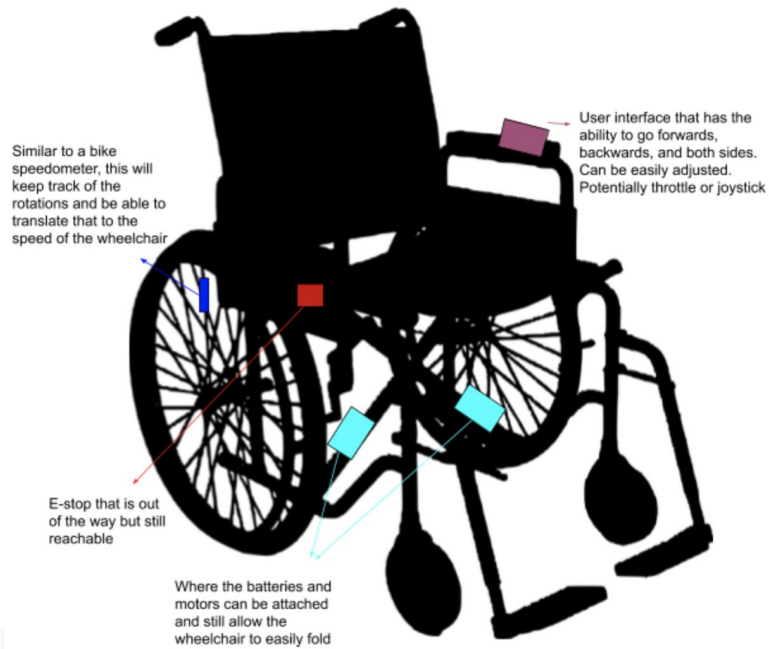
Figure B.9 Option for where we can place batteries, Estop, user interface and speedometer [25, modified]
