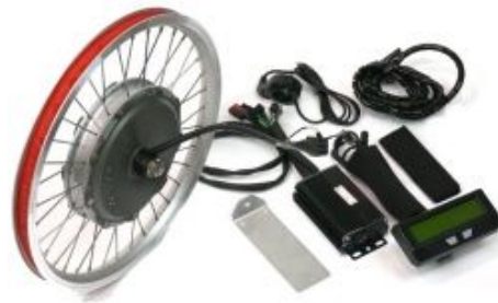
Figure A.2 Hub Motor in E-Bike Wheel [10]
