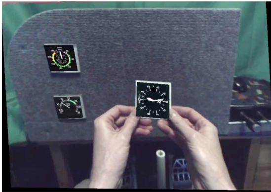
Figure 11. Detection of ArUco tags and overlay with simulated VR gauges. Moving counter-clockwise from the bottom left, ArUco tag identifiers 0, 1, and 2 are overlaid with the tachometer, altimeter, and air speed indicator.
