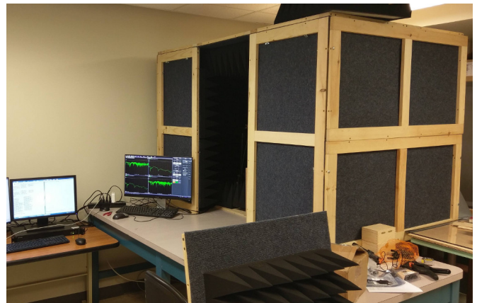
Fig. 2. Compact anechoic chamber used for measurements. The side panel is removed for easy positioning of the material and replaced for the measurement.
