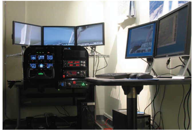
Fig. 8. X-Plane simulator setup at Lafayette College, consisting of pilot cockpit (left) and instructor control console (right).
