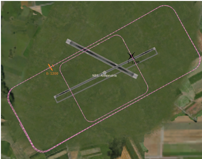
Fig. 6. Visualization of the flight paths for the first see-and-avoid study, generated by the X-Plane instructor console. The PAV (orange) is controlled by the computer to fly in a rectangular course. The drone UAV is shown in black. The path of the PAV and the desired path of the UAV are shown as magenta/white lines.
