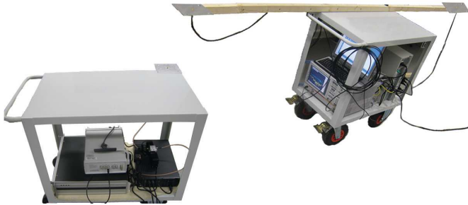
Fig. 2. Experimental setup of transmitter (left) and receiver (right) for shadowing cross-correlation
