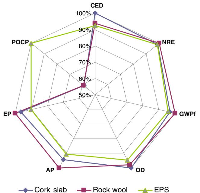
Fig. 5 Improvement scenarios: environmental impacts of pre-use and maintenance according to three types of insulation on the exterior facades
