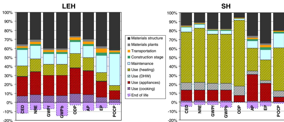
**Fig. 2** Contribution analysis of the life cycle subsystems. *LEH* low-energy house, *SH* standard house, *CED* cumulative energy demand, *NRE* non-renewable energy, *GWP<sub>f</sub>* global warming potential fossil, *GWP<sub>b</sub>* global warming potential fossil+biogenic, *ODP* ozone depletion potential, *AP* acidification potential, *EP* eutrophication potential, *POCP* photochemical ozone creation potential
