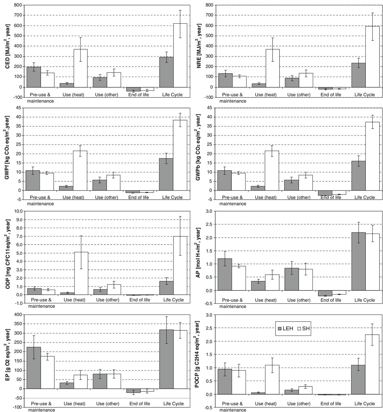
**Fig. 3** Comparison between the life cycle phases of the LEH and SH. (LEH low-energy house, SH standard house)
