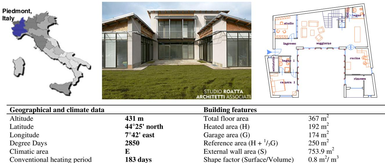
**Fig. 1** Main features and climatic data of the house in Morozzo
