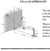
The shear leg derrick is to be designed to lift a maximum of 500 kg of fish.
