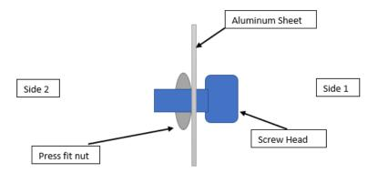
For the electronics panels ensure they are mounted on the inside of the enclosure, not the outside. As the panels are internally mounted for waterproofing purposes.
