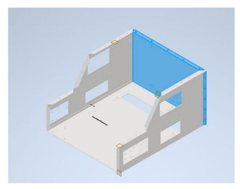
The screws heads should be on the outside of the enclosure. The back panel wraps around the sides. The sides are outside of the bottom panel.
