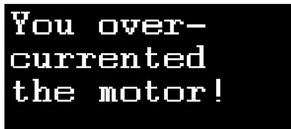
Figure 5: This is the overcurrent warning which is defined as warning number 2
