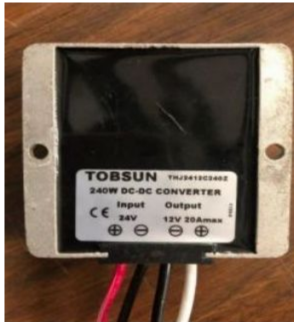
Figure 2 - 24V DC-to-DC Converter
