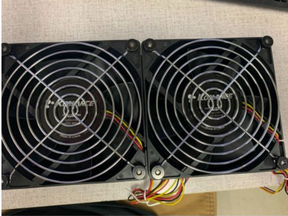
Figure 4 - Koolance fans mounted to radiator
