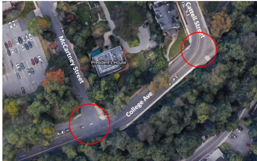
Figure 9: College Ave and McCartney Street Intersection. Note the sharp turn and lack of crosswalks.
