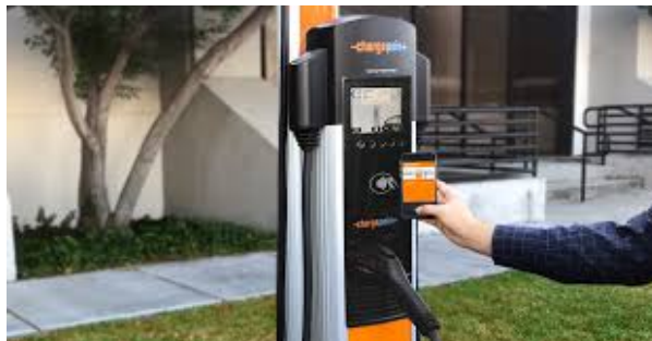
Figure 10: “Level 2 Charging Station”, (Chargepoint, 2019)
