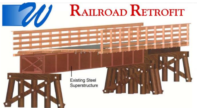
Figure10: Structure of the existing bridge (Reeve, Messer, Kulback, & Smith, 2016)
