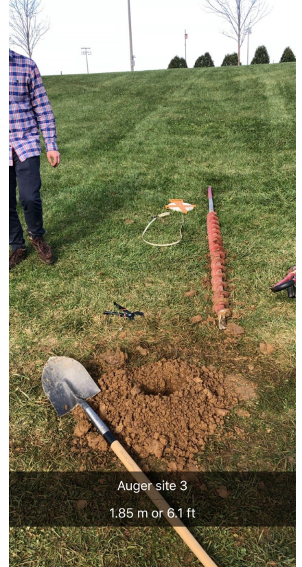
Auger Site 3 - Impermeable Layer Hit at 1.85 meters
