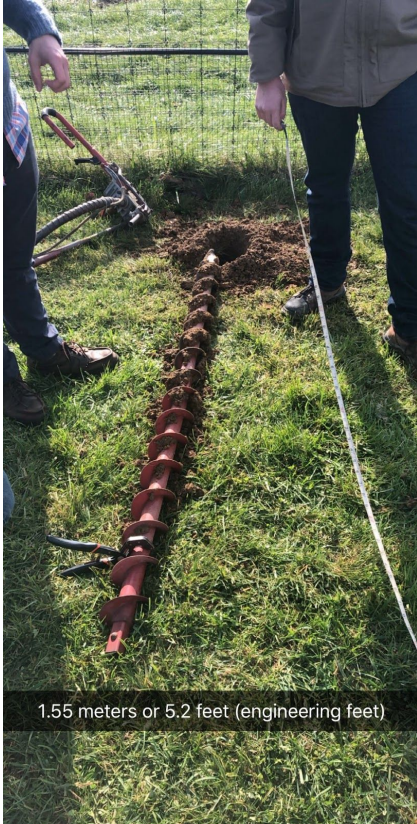
Auger Site 1 - Impermeable Layer Hit at 1.55 meters
