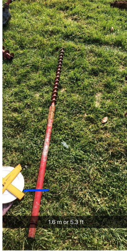
Auger Site 2 - Impermeable Layer Hit at 1.60 meters
