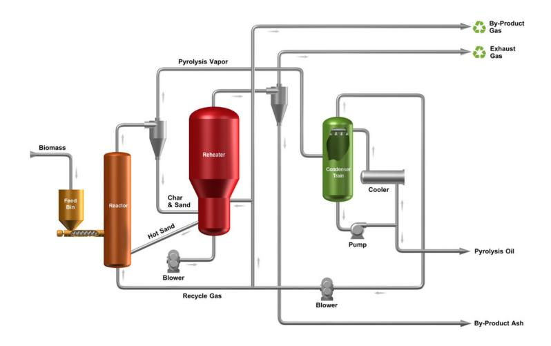
Figure 7: RTP Process Diagram (Source: Ensyn Technology Overview, 2015)
