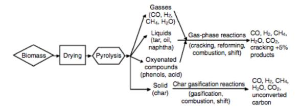
Figure 4: Potential Paths for Gasification (Basu, 2010 p. 119)
