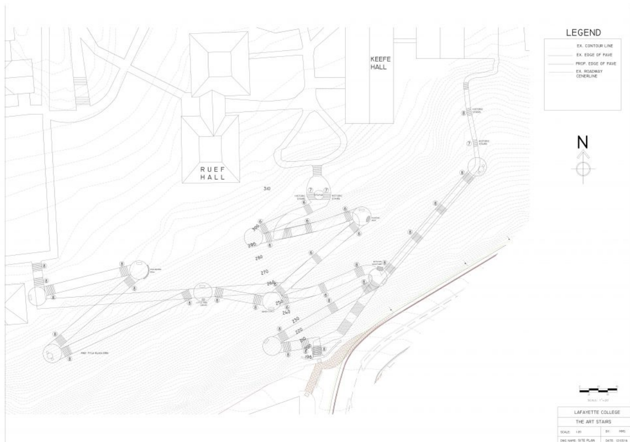
Figure 2: AutoCAD Drawing of new stair design, including the existing outline of stairs (See Figures 3, 10, 11, 12 for details on specific features).
