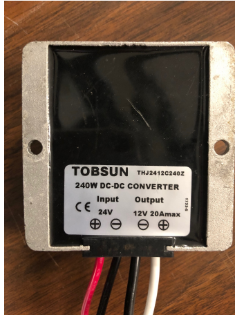
Figure 4 24v DC/DC converter
