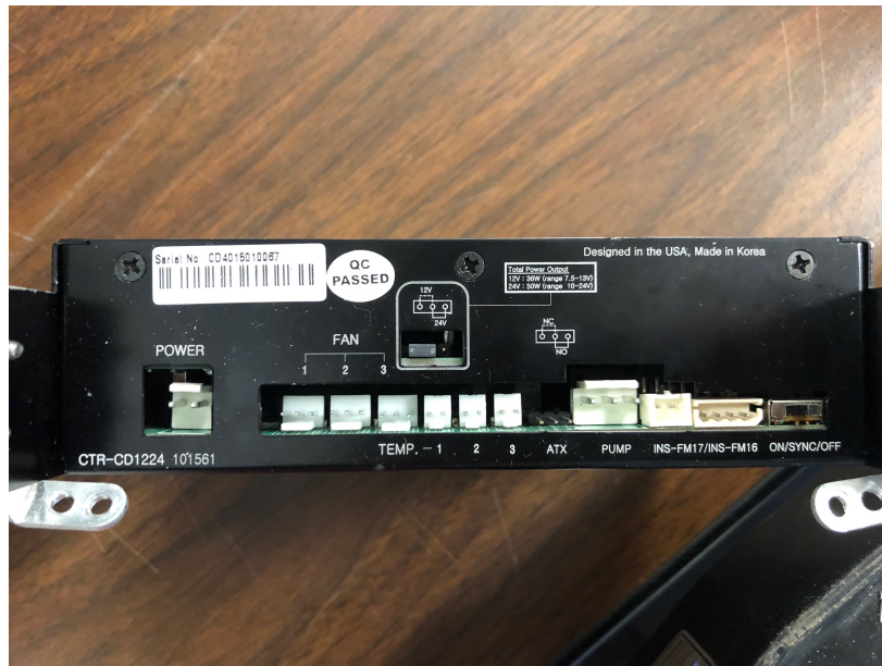
Figure 3 Cooling Controller Connections
