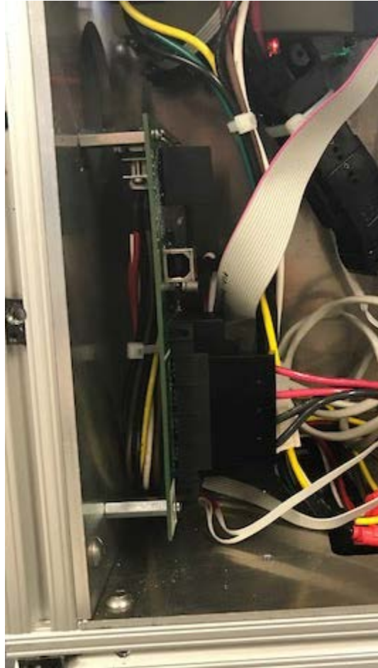
Figure 7. Installed Power Connector. LCD should turn on, AMS boards should ACK the PacMAN, Power LED should be on on the PacMAN, Heartbeat LED should be blinking. You have now successfully installed a PacMAN board into a pack.
