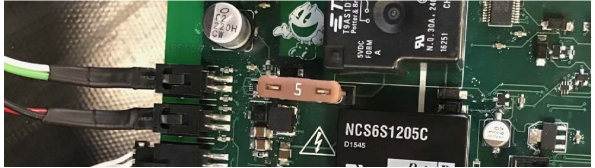
Figure 3. Installed Charge, LCO, and AMS connectors.
