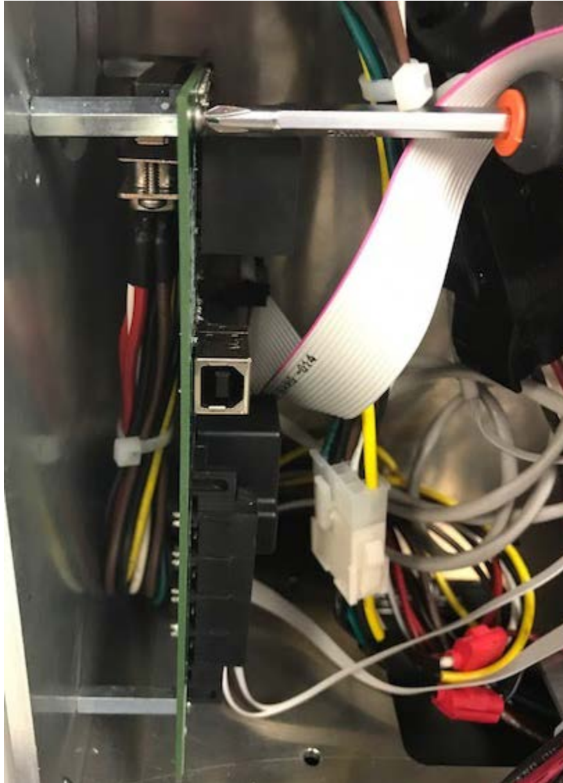
Figure 6. Install PacMAN into the Pack using the four 4-40 x 1/4 Button Head Socket Cap Screw screws and the Phillips Head screwdriver. The screws are to be screwed into the 4 standoffs mounted on inside side panel beneath the LCD.
