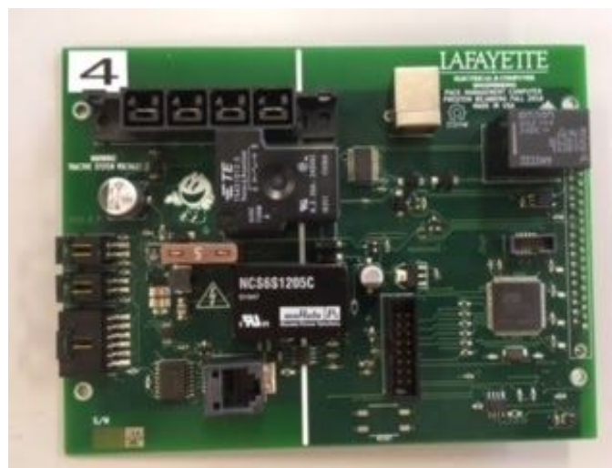
Figure 5. PacMAN Board (rev 0.8) that was utilized in the delivered accumulator system in the LFEV 2017 Spring semester. Pulled from Pack 4.
