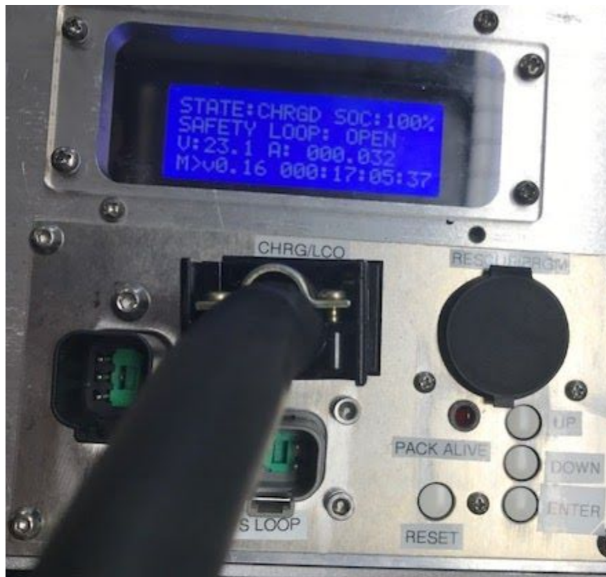
Figure 16. Charger plugged into pack and pack display indicating charging state. In this case, the pack has been 100% charged; therefore, the state reads “CHRGD”.
