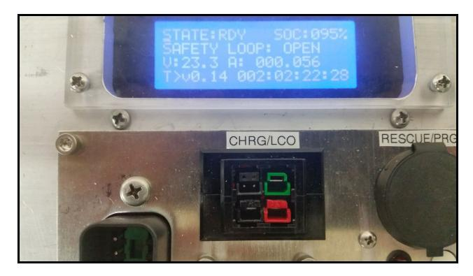
The port labeled CHRG/LCO is the Anderson port used for charging and low current output. It's female signal pins should be jumped to indicate charging. A charge cable should have its male pins jumped to accomplish this.
