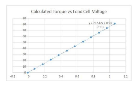
The calibration factor determined for this data has been incorporated into the proejct's legacy VSCADA software for purposes of data logging, and therefore measurements for the purposes of ATP items should be accurate to the standard set by a voltmeter.
