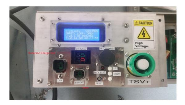
To charge, the charger should be plugged in and the "PREV" button with a lock icon next to it should be pressed. Then, adjust the knobs on the charger to set the voltage no higher than 28V and 20A; once this is done, the "OUT" button can be pressed to begin charging. Charging is plug-and-forget. The accumulator will stop charging automatically when the charge cycle is complete.
