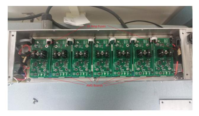
Shutdown for short term storage is accomplished by removing both of these fuses. For long term storage, to prevent any current from being drawn from the cells, all the fuses and all AMS boards may be removed.
