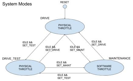
DRIVE\_TEST and MAINTENANCE states do not require a closed safety loop for operation. Transitions to MAINTENANCE require a password to be entered. A working, closed safety loop is required to provide power to the motor controller in DRIVE. These states are set and stored by the Raspberry Pi 3. IDLE is TRUE when no TSV current is flowing in TSI or PacMan, and motor RPM is 0.
