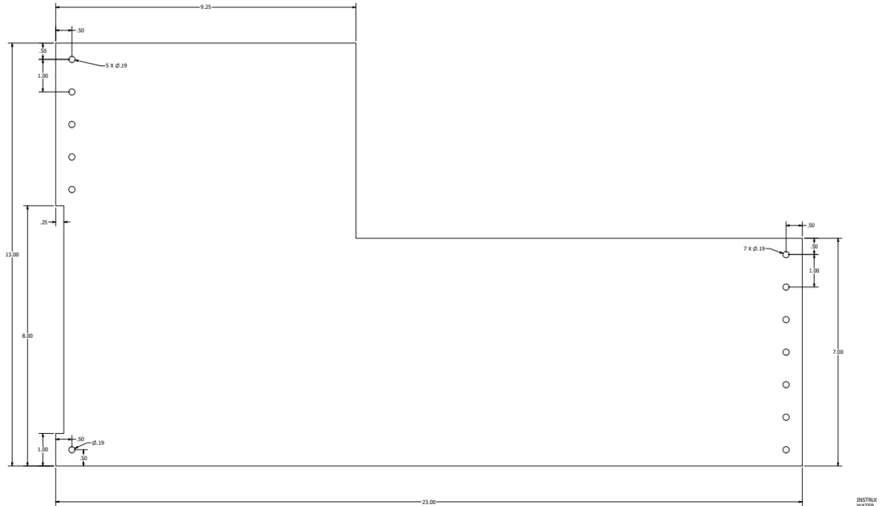
Fig 5: Modified power board with dimensions
