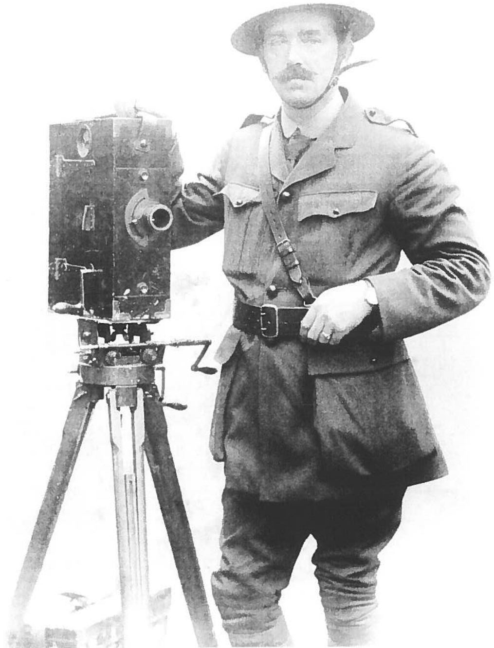
Fig 4 'Mac' McDowell with a Moy and Bastie cine camera as he appeared during the Battle of the Somme. The 'head' mechanism which traversed and elevated the camera can be seen on the tripod. While he moved the camera on the tripod with his left hand, the right hand had to maintain a steady two revolutions per second. Information from Kevin Brownlow in the book Ghosts of the Somme . British Film Institute
