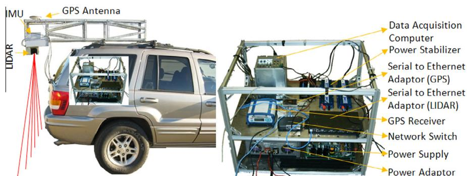
Fig. 2. Instrumented vehicle data collection system.
