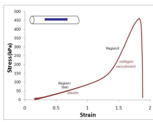
Stress-strain curve for bovine vein displays nonlinearity due to progressive recruitment of collagen fibers. Region I is dominated by elastin, while the steepening slope of Region II represents collagen's increasing contribution to vein's longitudinal stiffness.
