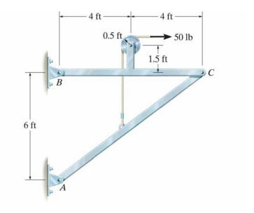
Find the internal shear force, normal force, and moment on bar BC at a location 2 feet from the pin connection at C
