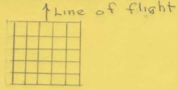
When a map is not available one can used a ground glass etched as a grid as shown in the sketch, a lens causes an image on the glass.
