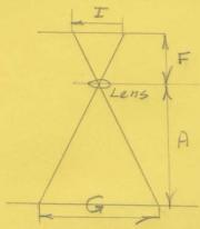
The diagram shows two similiar triangles. The lens of the camera converges the rays of light reflected from the earth.
