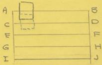
Flight lines are set up so that there is a side overap of photographs of 40%. (Theses lines are AB, CD, Etc. On the drawing) This overlap is easily computed as the altidude to be flown is known, the focal length of the lens is known and the size of the film is known. Therefore the the amount of ground covered can be computed as shown previously.
