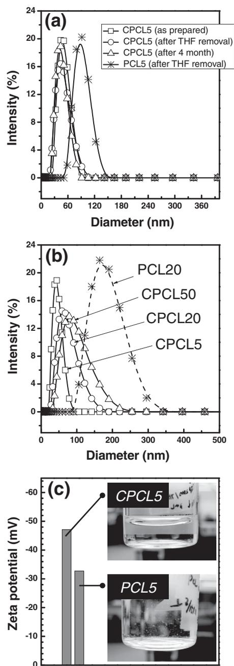
**Figure 4.** a) DLS plots of CPCL5 and PCL5. b) DLS plots of size-controlled nanoparticles (CPCL5, 20, 50) achieved by manipulating the concentration of CPCL in THF. c) Zeta-potential graph of CPCL5 and PCL5; inset images: CPCL5 and PCL5 nanoparticle aqueous solutions 4 months after nanoparticle preparation.
