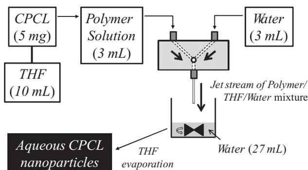
**Figure 2.** Schematic illustration of the preparation of aqueous suspended CPCL nanoparticles using the flash nanoprecipitation method.
