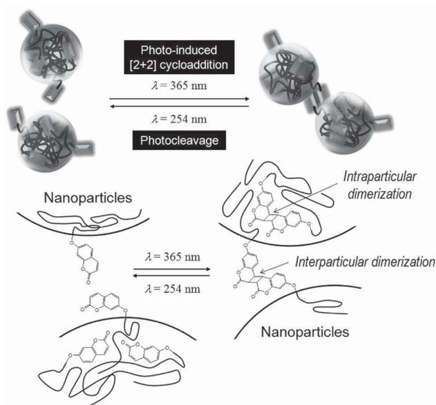
**Figure 6.** Schematic illustration of the photoresponsive behavior of CPCL nanoparticles by photoinduced [2 + 2] cycloaddition and cleavage of coumarin moieties in the nanoparticles.
