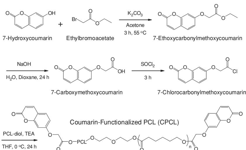
**Figure 1.** Synthetic scheme for coumarin-functionalized PCL (CPCL).
