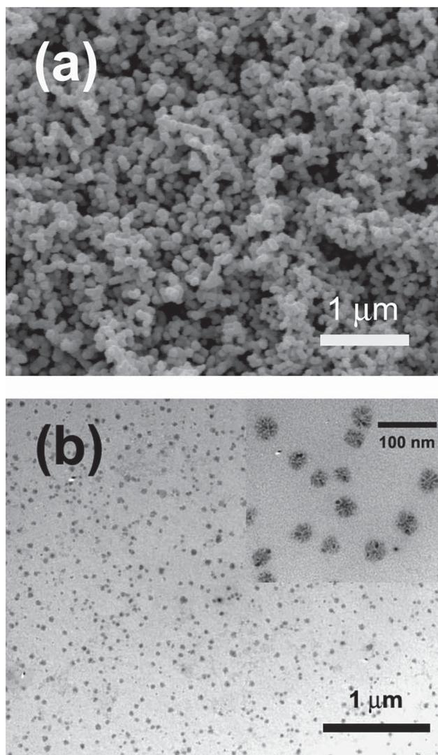
Figure 3. Morphology of CPCL5 nanoparticles visualized by a) FE-SEM and b) TEM.
