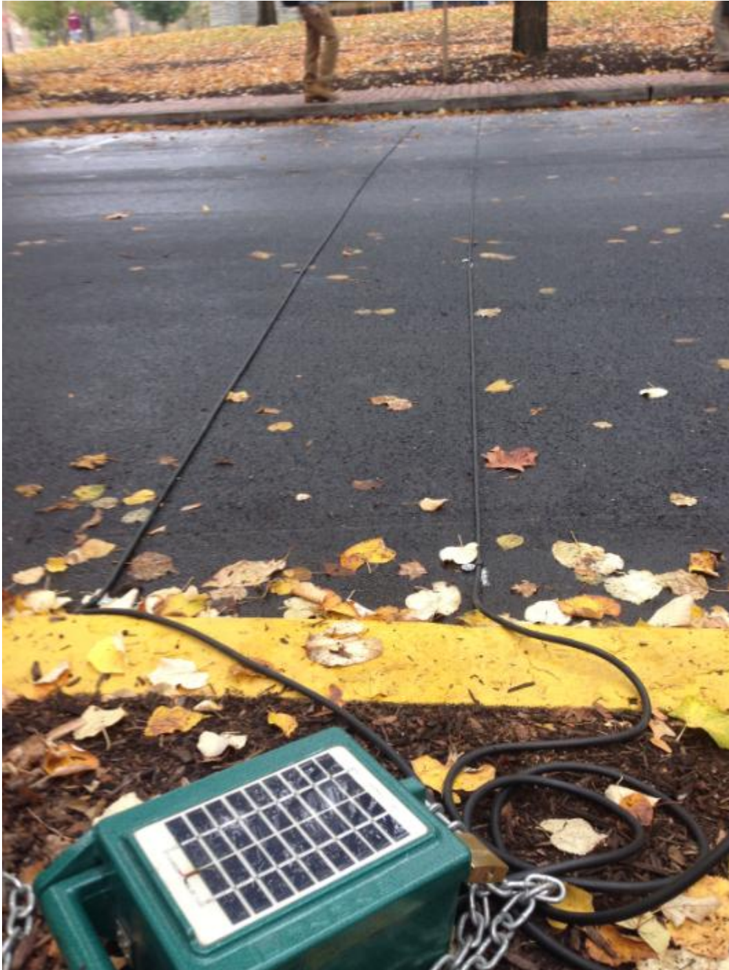
Figure F1: Pneumatic tubes and collector test setup on High Street [Photo taken by Josh Koerber]
