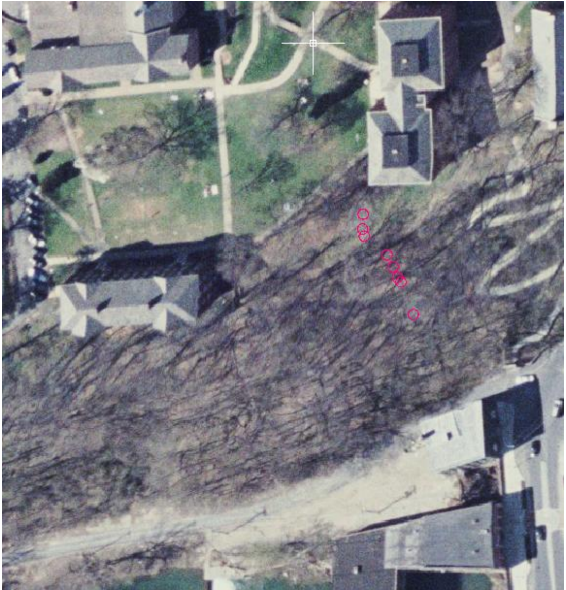
Figure E1. Boring Location Map. Pink circles indicate hand auger boring locations on the slope.
