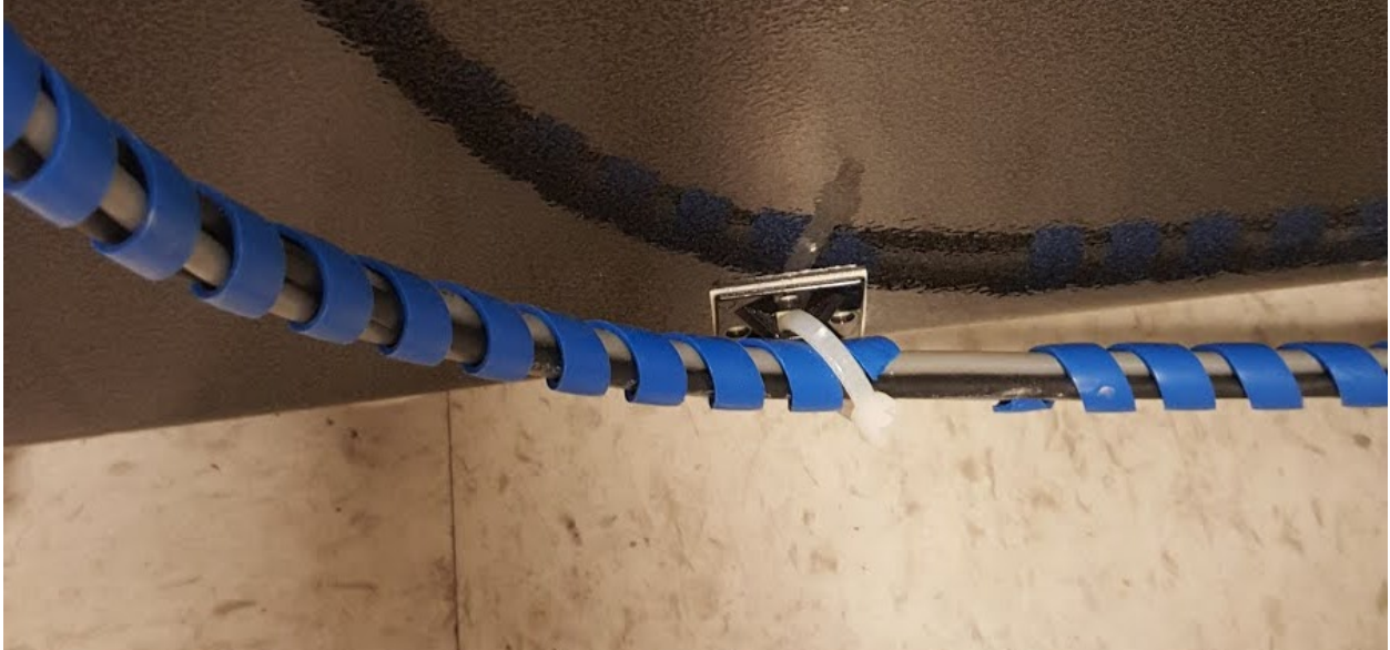
Mechanical strain relief for the sensor wires.
