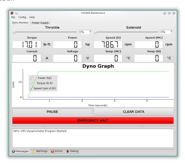
VSCADA provides the software solution for the DYNO system. With the VSCADA software, the user can turn the power supply on and off, monitor all of the sensor data listed above, control the throttle, and control the valve opening on the dynamometer.
