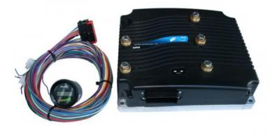
The Curtis motor controller provides, via CAN communication, motor velocity, motor controller temperature, output RMS current, motor temperature, and input voltage.
