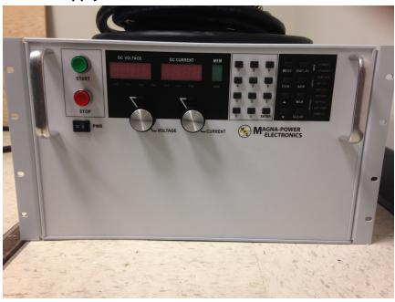
The power supply provides voltage and current sensors. We are able to read these values on the front of the power supply or through the dynamometer software.
