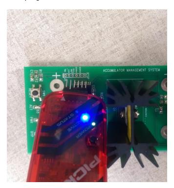
2. Connect the AMS board to the power supply.
