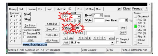
9. To test bypass mode, first increase the current limit of the power supply to 3A. This time, send the packet 0x01.
