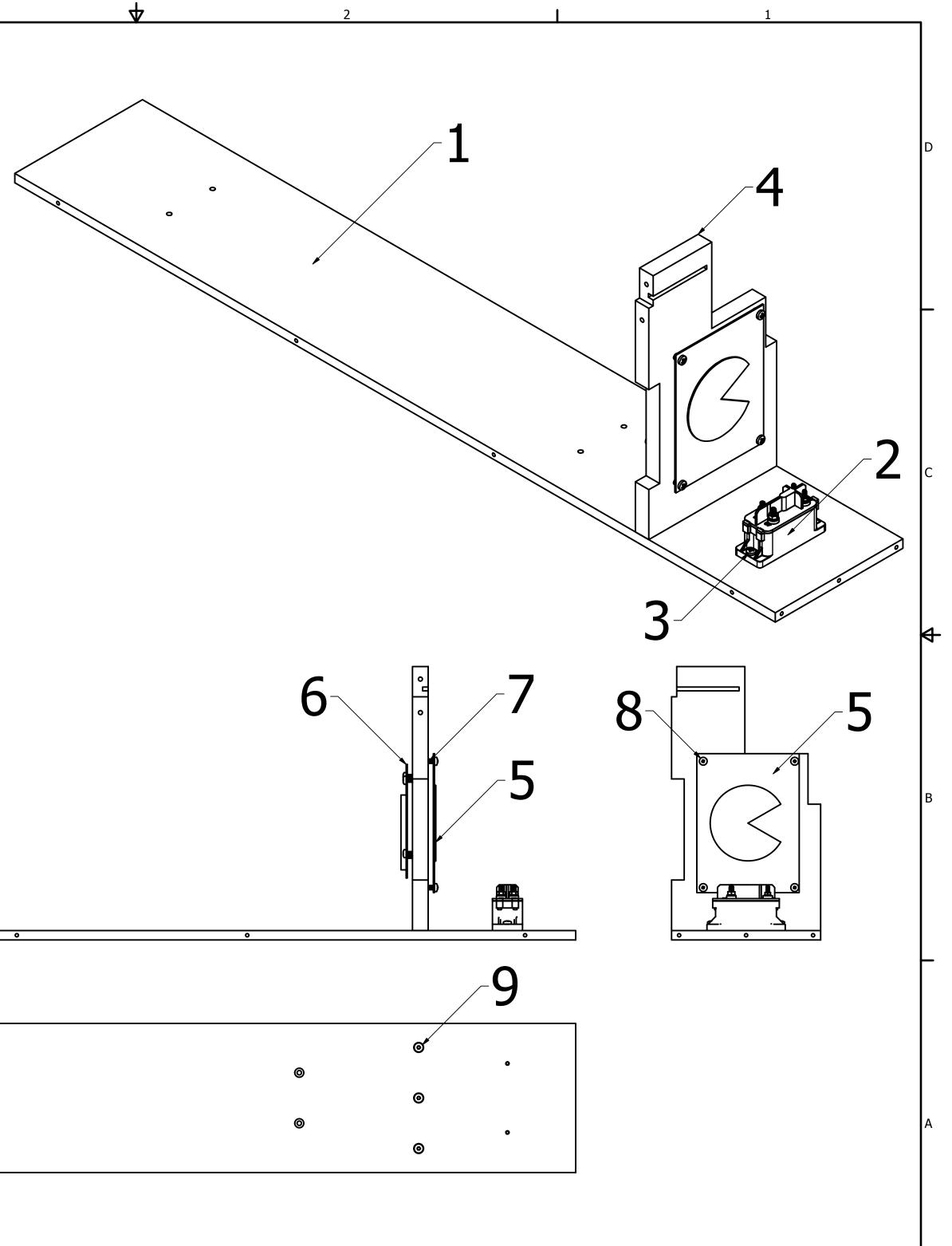
CONSTRUCTION NOTE: METAL STANDOFFS ASSEMBLED BY GLUING FEMALE SIDE UP AND MALE SIDE REMOVED
