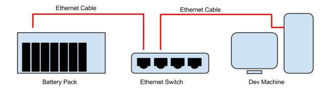
PacMan is configured to have the IP address of 192.168.1.51. Therefore, to access the board, ssh root@192.168.1.51
