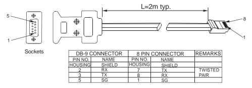
Fig.7-3: RS232 cable with DB9 connector (P/N: GEN/232-9)
