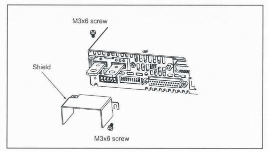
Fig. 3-6: bus-bars shield mounting
