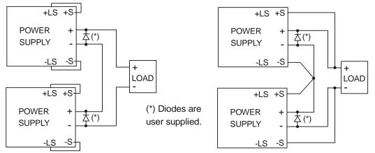
Fig.5-1: Series connection, local sensing
