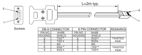
Fig.7-4: RS485 cable with DB9 connector (P/N: GEN/485-9)
