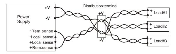
Fig.3-13: Multiple loads connection with distribution terminal
