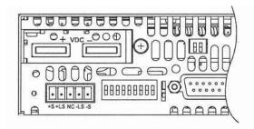
Fig.3-14: Sense connector location
