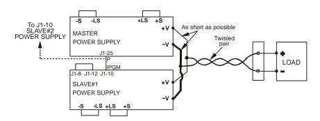
Fig.5-4: Parallel connection with local sensing
