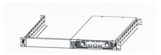
Fig. 3-1 Single unit installation
