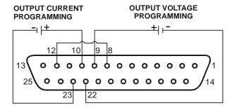
Fig.6-1: Remote voltage programming connection
