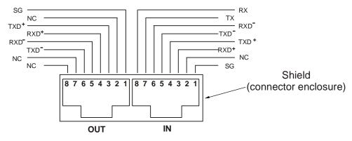
Fig.7-1: Rear panel J3 IN/OUT connectors pinout
