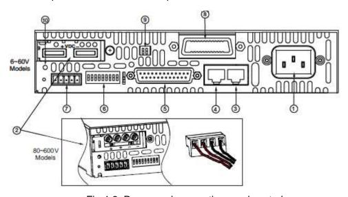
Fig.4-2: Rear panel connections and controls
