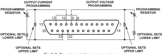
Fig.6-2: Remote resistive programming
