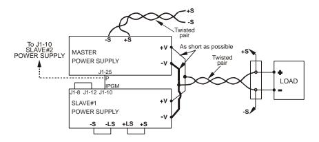
Fig.5-5: Parallel operation with Remote sensing
