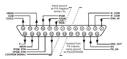
Fig. 4-4: J1 Connector terminals and functions
