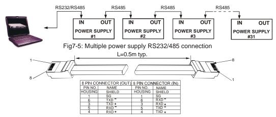
Fig.7-6: Serial link cable with RJ-45 shielded connectors (P/N: GEN/RJ-45)
