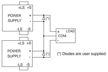
Fig.5-3: Series connection for positive/negative output voltages
