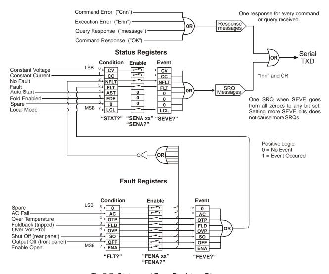
Fig.7-7: Status and Error Registers Diagram
