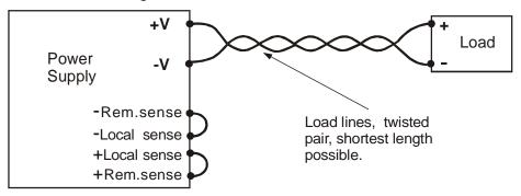
Fig.3-10: Single load connection, local sensing
