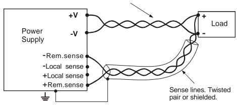
Fig.3-11: Remote sensing, single load
