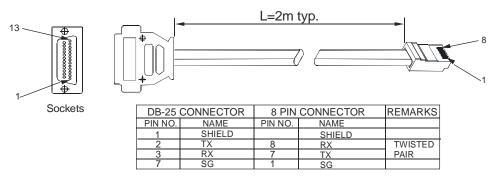
Fig.7-2: RS232 cable with DB25 connector (P/N: GEN/232-25)
