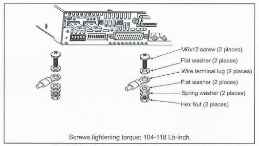
Fig. 3-5: Load wires connection, 6V to 60V models.
