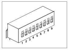
Fig.4-3: SW1 setup DIP-switch
