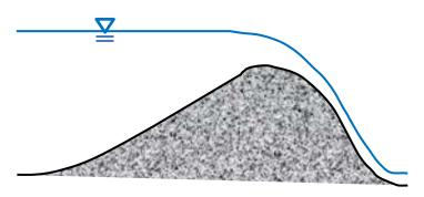
(a) To reproduce the field conditions using a 3-ft wide scaled model of the dam in our hydraulics laboratory, what flow rate of water (70°F) should we use? Give answer in cfs
