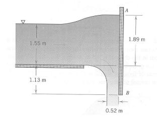
$Fw_x = 22.1 \text{ kN per m of width (to the right)}$
